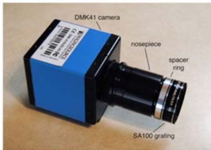
Figure 1. A simple converging beam slitless spectrograph can be created with the addition of a screw-in transmission grating before a camera.
