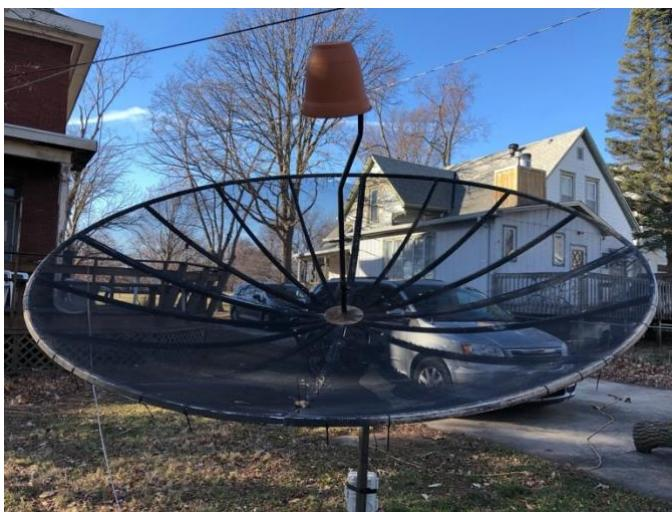
These simple radio telescopes are perfectly capable of receiving 21cm signals from cold neutral Hydrogen (HI)
