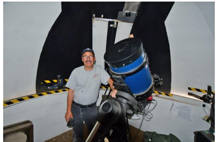
Inside the Hidden Valley Observatory's 10' dome is a nice 12" LX200 SCT, which is equipped for imaging and to provide views of celestial objects on a TV screen for visitors. In this photo is Rick Van Ness, the observatory director.
